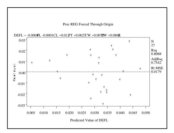
Figure 1. Residual Plot of Defect Loss Model for the Recommended Minimum Hardwood Cant Grade Rules.
