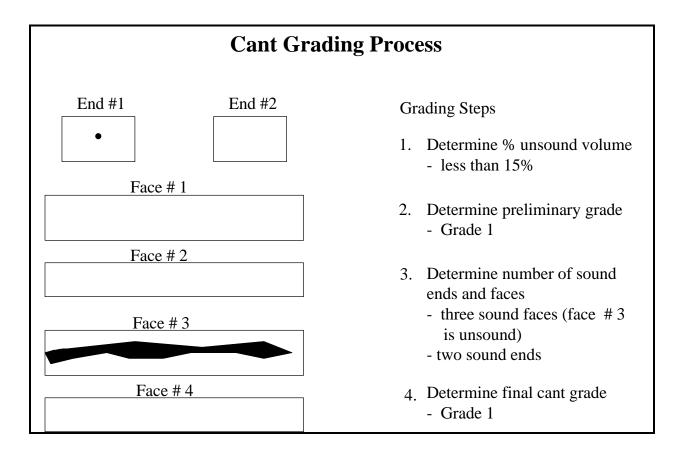
Figure 5. Schematic Diagram Showing Allowable Defects in a Grade 1 Hardwood Pallet Cant
