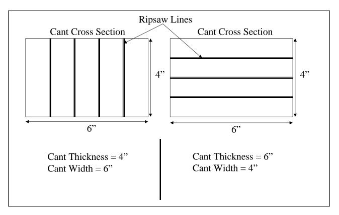
Figure 14. Schematic Diagram Showing the Different Sawing Orientations for a 4" X 6" Hardwood Pallet Cant
