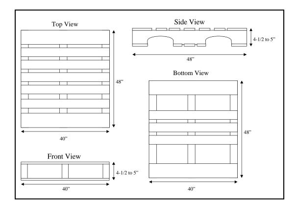
Figure 1. Schematic Diagram of 48" by 40" GMA Pallet
