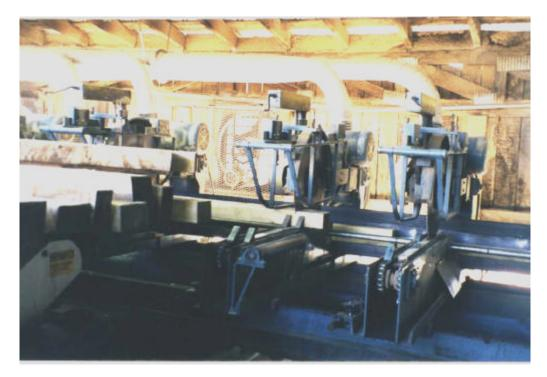
Figure 10. Hardwood Cants Entering the Trim Line of a Pallet Part Sawing System
