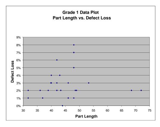
Figure 19. A Typical Plot of Defect Loss as a Function of Part Length for Grade 1 Cants
