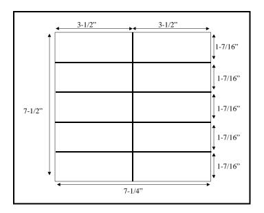
Figure 22. Ripsaw Sawing Pattern from Processing Hardwood Cants into Pallet Parts for Mill 23
