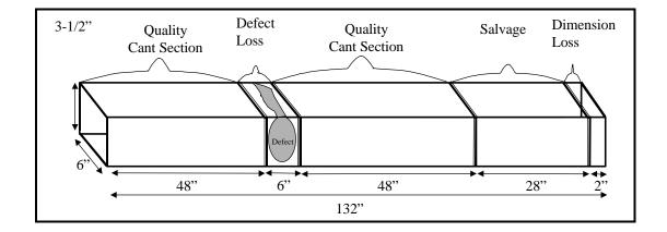
Figure 11. Schematic Diagram Showing Typical Defect and Dimension Trim Losses in Hardwood Pallet Cants
