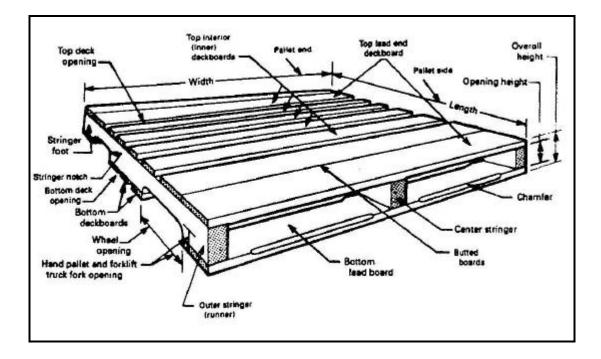
Figure 2. Schematic Diagram of Typical Stringer-Style Pallet (Source: ASME MH1.8M – 1996)
