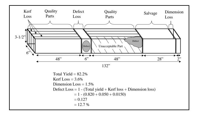
Figure 18. Defect Loss Calculation Example
