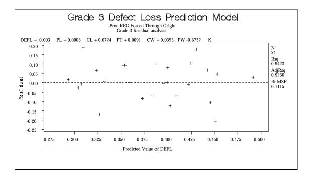
Figure 25. Residual Analysis for Grade 3 Defect Loss Model for Processing Hardwood Cants into Pallet Parts
