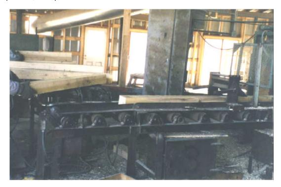
Figure 12. Quality Cant Sections Entering a Circle Gang Ripsaw in a Typical Pallet Manufacturing Plant
